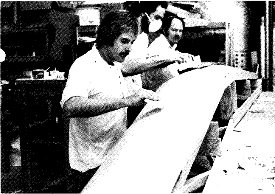
Applying the micro slurry mixture to the canard top surface. Note the jiggling so that the foam cores hold their shape.
