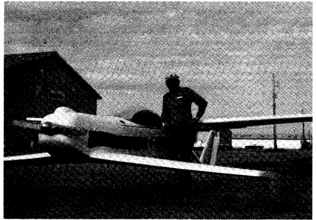
Garry LeGare and his big tire "Tundra" Quickie. The revised tires and wheels pants will be available as an option beginning 1 February, 1980. That package is but one of many that QAC is making available, including a 22 h.p. engine kit, Kevlar engine mount, and communications antenna kit.
