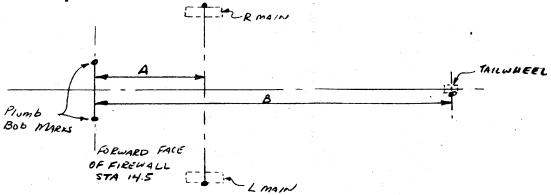
To get the moment arm (fuselage station) of the main gear add distance A to 14.5 (it should be about STA 42.3); To get the moment arm of the tailwheel, add distance B to 14.5 (it should be about STA /86.0).
